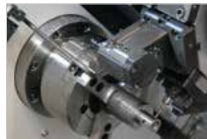
Chuck Air Blow (Upper Chuck)
