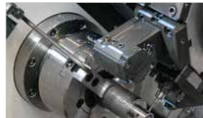
Chuck Air Blow (Upper Chuck)
