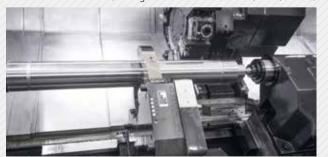
For long parts, such as shafts, the optional steady rest increases rigidity and minimizes vibration. When using the programmable hydraulic work rest provided as an option, the position of the work rest can be adjusted according to the shape of the product using the alignment pin connected to the turret. This enhances the efficiency of the machining operation.
