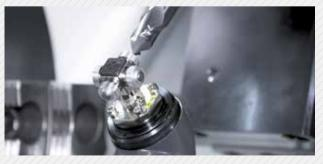
Cutting tools are calibrated quickly and accurately with the addition of a O-Setter.
